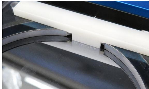
*Figure 5: Clamping Bar Installed*
