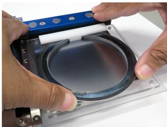
*Figure 6: Scribing a Wafer using Wafer Holder*
