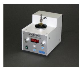
Micropol polisher is a compact, versatile, electrically controlled, precise mechanical specimen grinder/polisher designed for planar grinding, dimpling, thinning and polishing of specimens in the fields of nanotechnology, semiconductors and material science. The parameters of polishing (speed, load, time, etc.) can be matched according to the properties of the specimen. High quality samples are prepared with minimal efforts by the operator.
