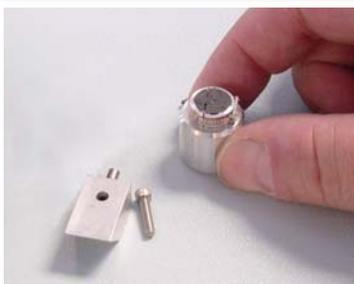
The PTR-2000 uses modified Fortress™ holders to securely hold samples in the FIB for processing and then directly transferred to the rod for processing in a plasma cleaner. If a low power plasma is used, then the sample can be exposed directly to the plasma without any
