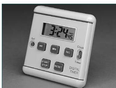
A six digit quartz timer with audible alarm, offering count down, count up and clock modes. The timer can be programmed for count downs of up to 24 hours, and includes count down memory recall, a pocket clip/stand and a magnetic mount.
