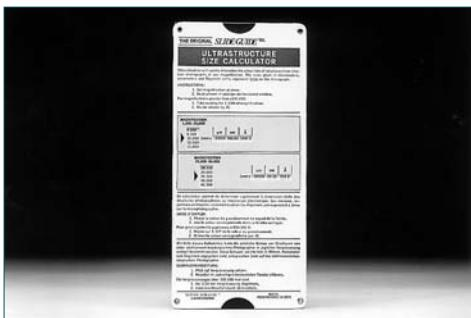
A simple slide rule calculator for determining actual sizes of structures from a micrograph, at any magnification.
