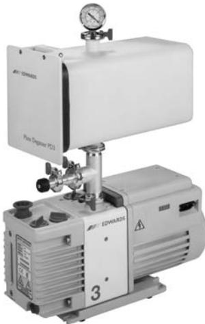
This simple, compact desiccator has a chamber designed to accommodate all types of film. Two chambers may be mounted on a T-piece if required, allowing cassettes to be used alternately. The pump has a non-return valve, allowing cassettes to be stored under vacuum when the pump is not running.
