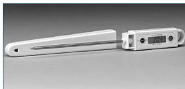
Battery operated digital thermometer with stainless steel probe. It has an operating temperature range of -50 to +150 °C, with an accuracy of ± 1 °C.
