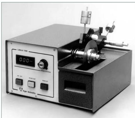
Low speed diamond saws offer convenient, precision cutting for a wide variety of materials in the laboratory, including mineralogical sections, embedded tissue, teeth, bone, semiconductors and other embedded devices. Low speed saws cause minimal damage and deformation of the sample and are particularly suited to fragile or soft materials.
