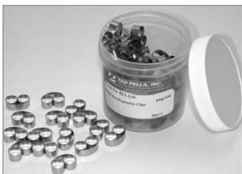
Metal clips ideal for holding thin samples during cross-sectioning. Can be used for hot and cold embedding.
