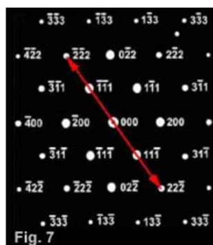
Fig. 6: Electron diffraction pattern from single crystal silicon, with the beam parallel to the [011] zone axis.
