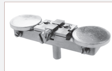
J402 TEM grid/sample holder, 2 sample pucks, stainless steel
