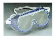
Multi-purpose safety goggles with polycarbonate lens to guard against impact eye hazards. Vinyl frame with soft border for excellent fit, adjustable head strap. Perforated for added ventilation and comfort. Sold in packages of 6.
