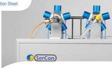
The deuterium and oxygen-18 signature of a water based sample is measured by equilibrating with hydrogen and carbon dioxide respectively. A procedure that is totally automated and allows either separate or sequential analysis of the two isotopes.
