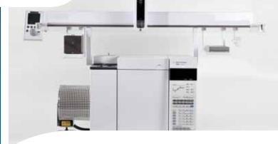
reaction Poraplot-Q or Molsieve 5a open tubular column may be used to separate analyte gases from minor bi-products of thermal decomposition dependant on configuration.
