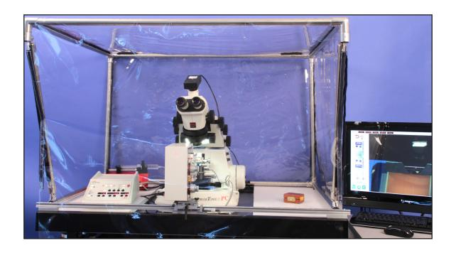
**Location (room):** suggest 8ft x 8ft (2.5m x 2.5m) minimum Free of air drafts (draughts) and temperature fluctuations. Air conditioning ducts should be located to avoid directing air onto the equipment.
