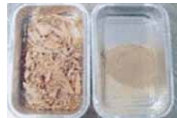
Wood: 50ml steel jar/ 20mm steel ball 200 Micron after 90 seconds.
