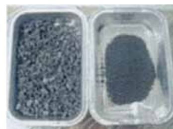
Rubber: 50ml steel jar/20 mm steel Ban after cryogenic grinding.
