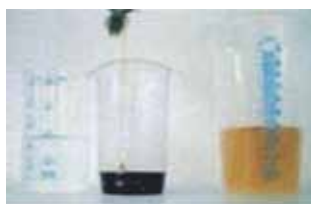
Honey/Water: 160ml steel jar/Static Mixer Homogeneous Mixture.
