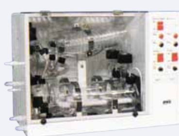
Double Distillation Aquamatic Stills AWC/4D - Output approximately 4 Liters per hour of high purity distillate. Four silica heaters.
